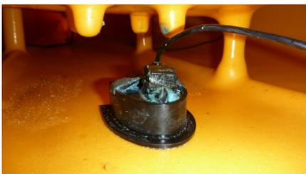
As for mounting the battery. I purchase an additional Hobie gear bucket and use the rear hatch to store my 12-volt battery. An X-acto knife was used to cut out the center rib and a Minnkota waterproof circuit breaker was purchase to use as my fuse. I extended the wiring and I am very happy with the use of the rear hatch for the battery storage. Here's a photo of the finished installation of the 12-volt battery.
